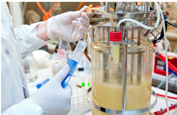
Bioreactor which contains live culture for chemical synthesis. (source: Shutterstock)
